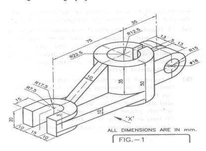
b) Draw the isometric view of the object, the orthographic views of which are shown in the figure below.
